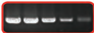
Gel image shows exceptional sensitivity of Accuris™ Hot Start Taq Polymerase with 405bp plant mitochondrial DNA. Amplification was performed with decreasing amounts of starting material, from 500ng to 31.25ng.
